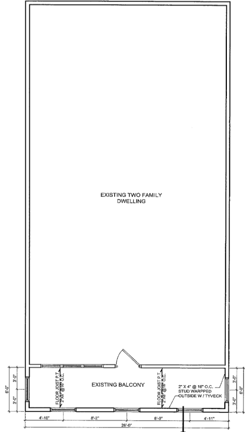
2nd FLOOR BALCONY PLAN SCALE: 1/4" = 1'-0"
